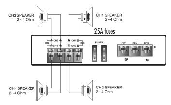
Note that the two speakers & four speakers have been connected to the four terminal following the (+) and (-) graphic. Your speaker terminals may be marked (+) and (-) or there may be red dot by one terminal which means the same as (+). Connecting the speakers in this manner assures that the two speaker cones will move in and out together according to the original recording. If one of the two speakers is reversed, stereo imaging and bass response will be degraded.
